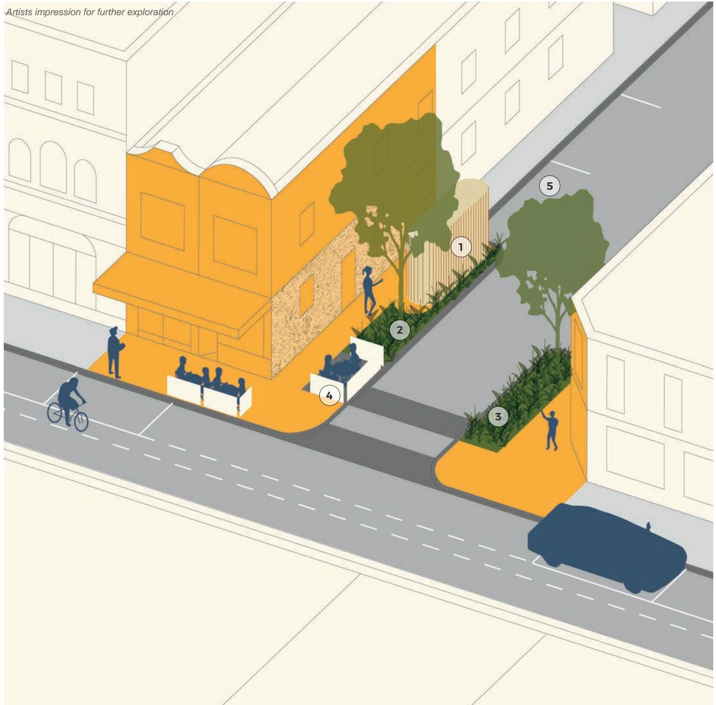
① Placement of public bathroom. This will require the removal of one 15 minute parking space and extension of the outstand kerb. Facade treatment to be designed. Access doors on the footpath side of the structure
